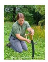
A blunt tool will not do the job it is designed for and could be unsafe, as it can result in the user having to apply extra force. Therefore, it is essential to learn the correct method for sharpening and keep blades sharp.
